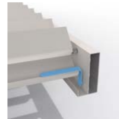
Algarve Line can drain an amount of water equivalent to rains with an intensity of between 144 mm/h and 180 mm/h that last up to 2 minutes maximum. These kinds of rains occur on average once every 10 years in Belgium. (See Belgian rain statistics: NBN B 52-011 norm)
