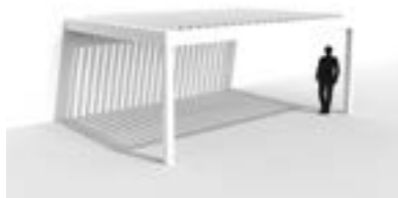
Fitted to an outside wall: the frame is placed with one or two sides against an underlying, supporting construction or structure. Vertical columns support the other part. The blades can be positioned parallel or perpendicular to the support structure.
